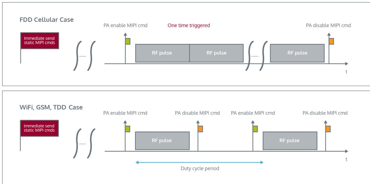
Synchronized MIPI testing is a challenging procedure. The time gap between the MIPI command and the RF pulse should be almost negligible. The DIO connector and the RF signal synchronize automatically through the same FPGA. The auto synchronization is successful with burst and modulated RF signals.
